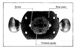
Secure the templet to the workpiece. Place the tool on the templet and move the tool with the templet guide sliding along the side of the templet.
